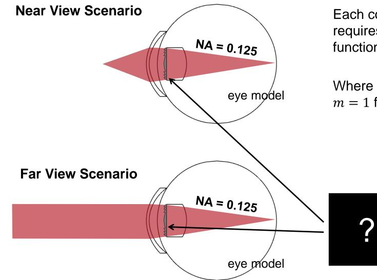
Each configuration of the two intraocular lens requires a certain wavefront phase response function.
